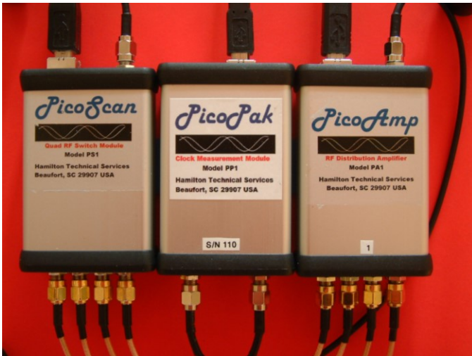
Figure 6. Coherent Test Setup for a 4-Channel PicoScan Clock Measurement System
